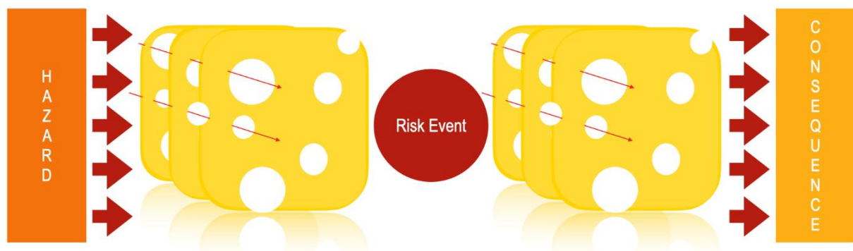
Figure 1: Example of Bow Tie Model Analysis with Swiss Cheese Model - adapted from SRMBoK (Talbot & Jakeman, 2009)
